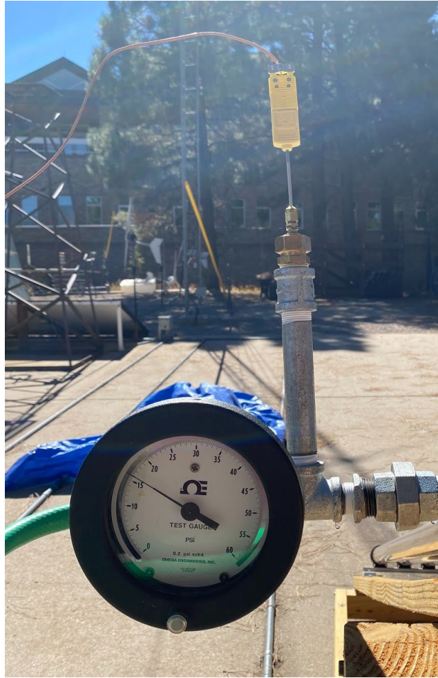
Figure 2. Barometer and thermocouple at inlet during test
